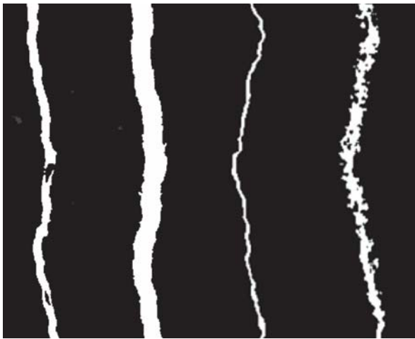
Fig.2 A cross-section of the fracture. From left to right: (1) 100% carbonate before dissolution, (2) 100% carbonate after dissolution, (3) 85% carbonate before dissolution, (4) 85% carbonate after dissolution
