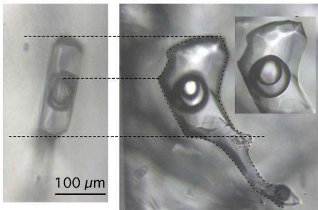
**Figure 1.** Three-phase carbonic inclusion according to two perpendicular sections
