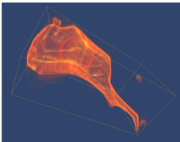
**Figure 2.** Image of the inclusion shown in Fig. 1 obtained using 3D X-ray microtomography
